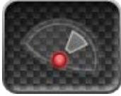
When you launch the application, the a-GPS will pre locate you via triangulation on the cellular network. The precision is low and can vary quickly. The dish shows you a moving sector.
